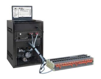
The EVd-40 can discharge batteries at high power (10,000 watts). **A Prius battery subjected to this** discharge power will exceed initial currents of 40 amps.
