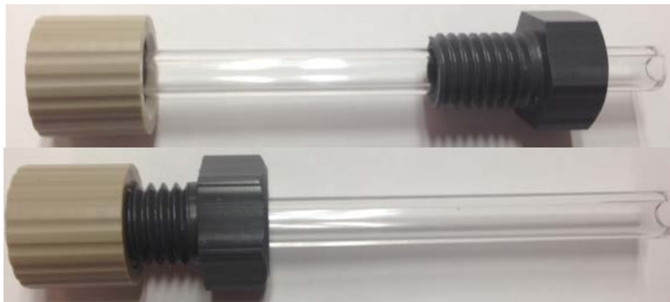
Figure 4. Assembly of bolt into seal piece
