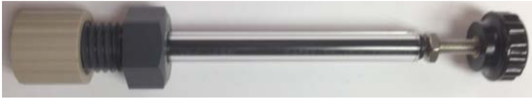
Figure 6. Placement of stainless steel rod into seal piece
