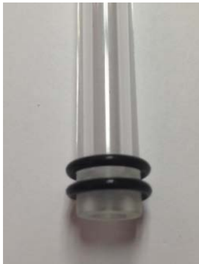
Figure 2. Glass rod with o-rings attached at ground end.
