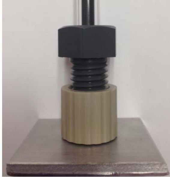
Figure 10. Placement of electrode into coupon
