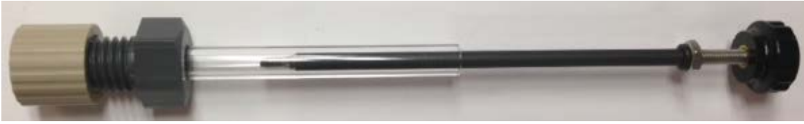
Figure 5. Placement of stainless steel rod into glass rod
