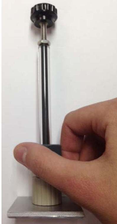
Figure 12. Forming the o-ring seal with the coupon
