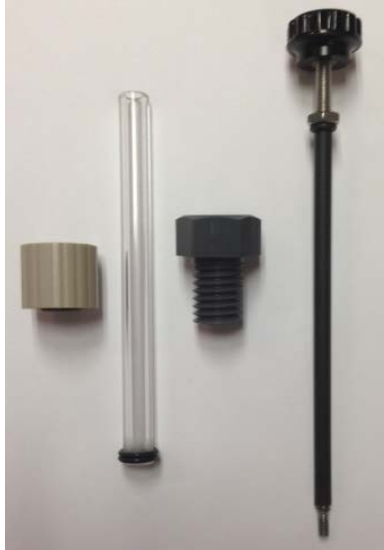
Figure 1. From left: PEEK piece, glass rod (with o-rings), bolt and stainless steel rod
