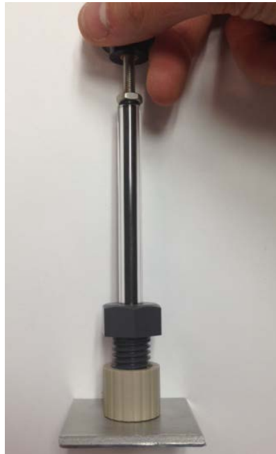
Figure 11. Initial attachment of electrode mount into coupon
