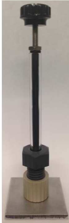
Figure 13. Electrode mount attached to coupon
