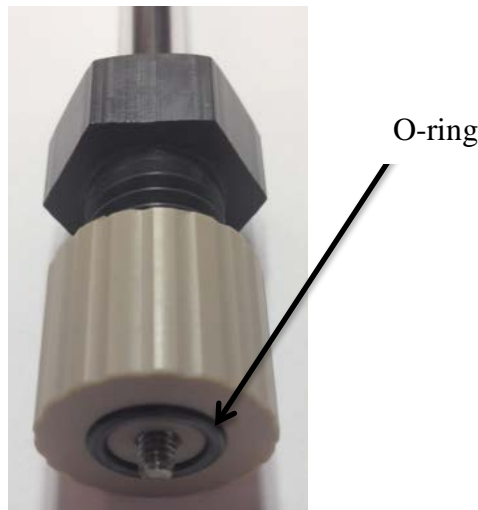
Figure 7. Protrusion of stainless steel rod through bottom of PEEK piece
