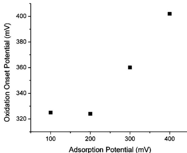
Fig. 9. CO electro-oxidation onset potentials vs. adsorption potentials.
