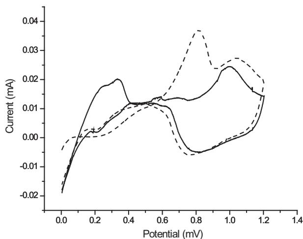
Fig. 6. Cyclic voltammetry (10 mV/s) of fuel cell working electrode (5-cm<sup>2</sup> geometric) under humidified nitrogen at 50 °C (solid). Humidified  $\text{H}_2$  (50 sccm) at the counter-reference. CO stripping wave (dashed).
