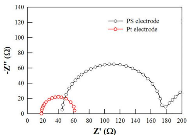
4 Nyquist plots of the PS and Pt electrodes under zero voltage bias over a frequency range of 0.1 to 100,000 Hz
