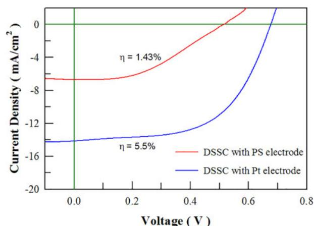
3 J-V curves of the DSSCs with PS counter electrode and the Pt counter electrode under the illumination of one sun
