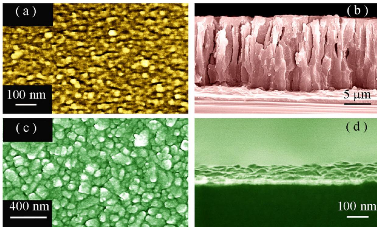
2 Top and sectional SEM micrographs: *a, b* the PS counter electrode; *c, d* the Pt counter electrode
