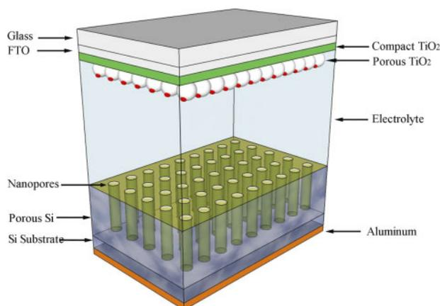
1 Schematic illustration of the structure of a DSSC with PS counter electrode
