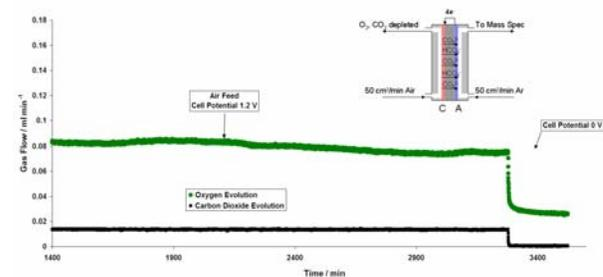
**Figure 3.** Long term air separation shows the extensive concentration of carbon dioxide from the air that is possible. The resulting gas stream is 15% CO<sub>2</sub>.
