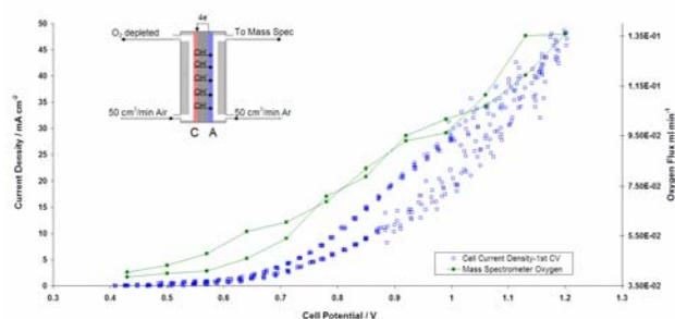
**Figure 1.** Current density and oxygen readings taken at the anode confirm oxygen separation from the air at potentials lower than 1.0 V.
