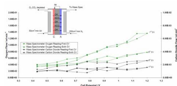
**Figure 2.** Oxygen evolution decreased as the cycles increased. Carbonation of the electrolyte occurred which resulted in the separation of both oxygen and carbon dioxide from the air.
