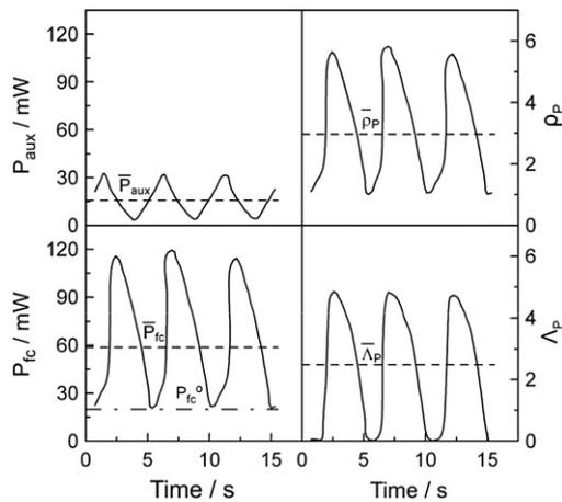
**Fig. 5.** Time variation of fuel cell power output,  $P_{fc}$ , sacrificed power in the auxiliary cell,  $P_{aux}$ , power enhancement ratio,  $\rho_p$ , and power gain ratio,  $\Lambda_p$  and corresponding time-averaged values for triode operation during imposition of a cyclic auxiliary potential,  $1.0\text{ V} \leq -\Delta V_{aux} \leq 1.9\text{ V}$ , under a fixed external resistive load ( $R_{ext} = 0.5\ \Omega$ ). Anode feed: 50 ppm CO/H<sub>2</sub>.
