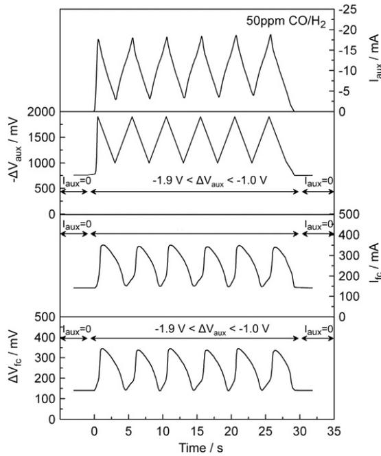
**Fig. 4.** Effect of a cyclic auxiliary potential application,  $1.0\text{ V} \leq -\Delta V_{aux} \leq 1.9\text{ V}$  on the auxiliary current  $I_{aux}$  and on the cell potential  $\Delta V_{fc}$  and cell current  $I_{fc}$ , under fixed external resistive load ( $R_{ext} = 0.5\ \Omega$ ). Anode feed: 50 ppm CO/H<sub>2</sub>.
