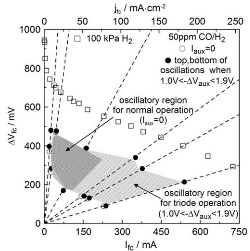
**Fig. 6.** Effect of cyclic auxiliary potential application ( $1.0\text{ V} \leq -\Delta V_{aux} \leq 1.9\text{ V}$ ) on the limits of fuel cell current-potential oscillations. The dark and light dashed areas show the region of self-sustained oscillations for normal and triode operation respectively. Anode feed: 50 ppm CO/H<sub>2</sub>.
