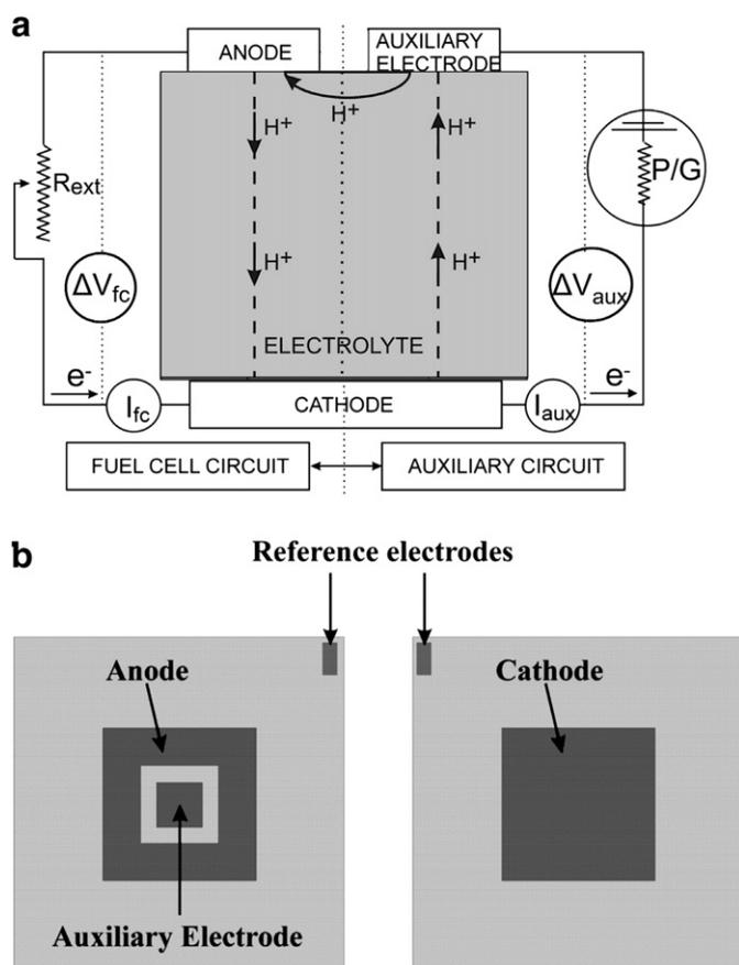
**Fig. 1.** Schematic of the triode fuel cell concept, showing the fuel cell and auxiliary circuit in detail (a) and the geometry of the membrane electrode assembly (b). The fuel cell cathode acts simultaneously as an electrode of the auxiliary circuit. P/G: potentiostat-galvanostat.
