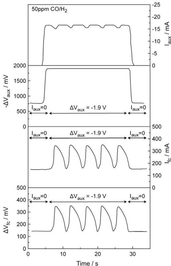
Fig. 3. Effect of a constant auxiliary potential application,  $\Delta V_{aux} = -1.9$  V on the auxiliary current  $I_{aux}$  and on the cell potential  $\Delta V_{fc}$  and cell current  $I_{fc}$ , under fixed external resistive load ( $R_{ext} = 0.5 \Omega$ ). Anode feed: Anode feed: 50 ppm CO/ $H_2$ .
