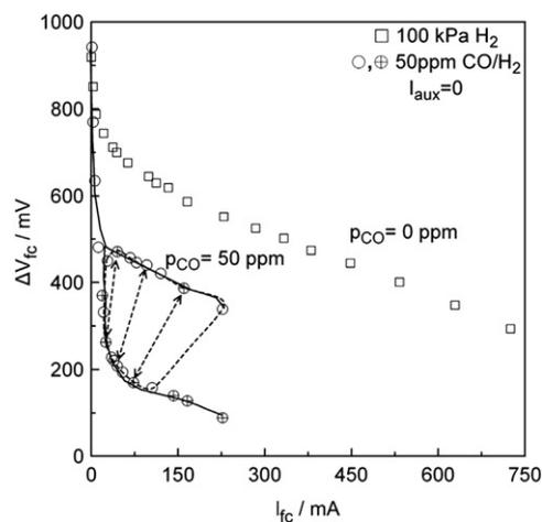
**Fig. 2.**  $I_{\text{fc}} - \Delta V_{\text{fc}}$  curves of the fuel cell circuit obtained with the conventional operation mode ( $I_{\text{aux}} = 0$ ) by varying the external resistive load,  $R_{\text{ext}}$ . Anode feed: 50 ppm CO/ $\text{H}_2$  (cycles).
